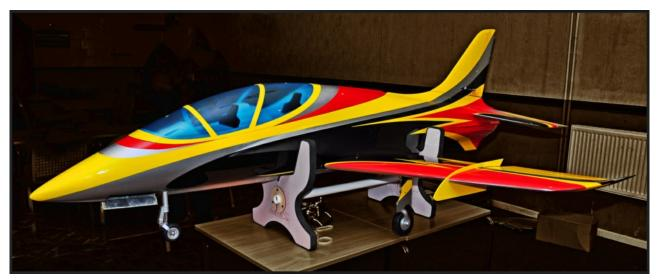
Mark Conlin brought his new Sebart model, the Avanti S. Another state of the art sleek jet but this time with vectored thrust. Mark said that it had presented many problems in mounting the jet engine - he had to make up jigs to be able to correctly align the motor within the very cramped space available. What he described to us sounded to have been a bit of a nightmare.
