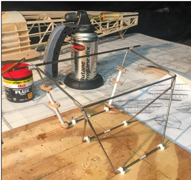
PIC 43 – Illustrates the undercarriage complete with wheels, which were secured using wire circlips made from 30amp fuse wire and steel washers, soldered to the axle. I used a thick tin foil baking tray to act as a heat shield to protect the plastic wheel hubs from the
