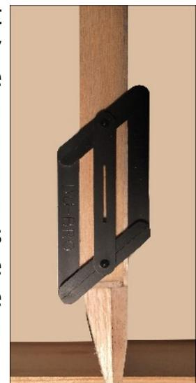
PIC 38 - The only problem was using a thinner blade meant there was a certain amount of freedom when cutting with a thin blade with the jig which is meant for a blade of 0.8mm however, it was a lot easier than having no guide and the slots cut in the wing trailing edge aligned a lot more
