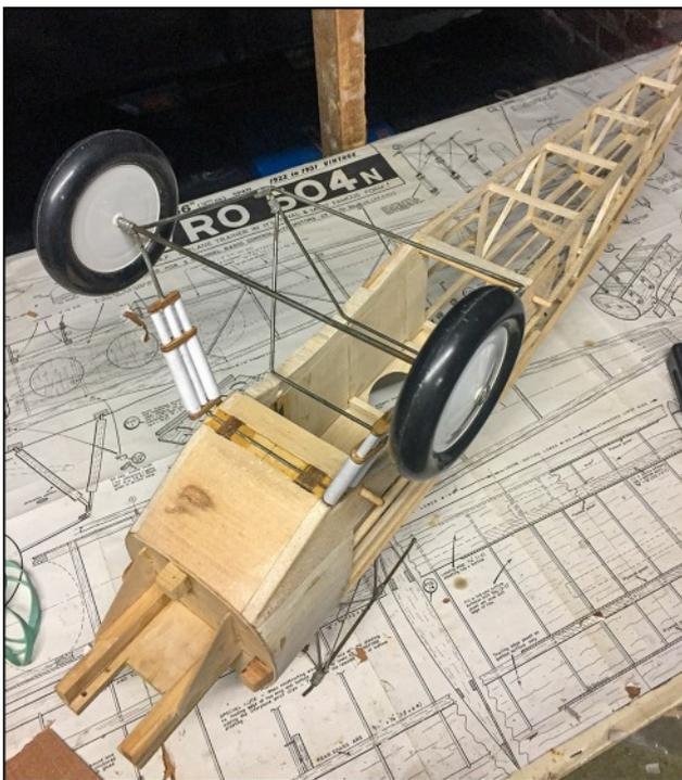
allow the undercarriage to be hinged to allow access and fitting of the wing. The elastic bands used to secure the wing also secures the undercarriage in slotted hardwood cross pieces in the wing.
