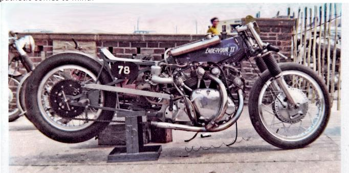
This was Dave's superb Vincent Shadow bored out to 1300 cc. 2 litre supercharger and modified 2½" SU carb with a 3mm main-jet, run on a mixture of methanol and nitro.
