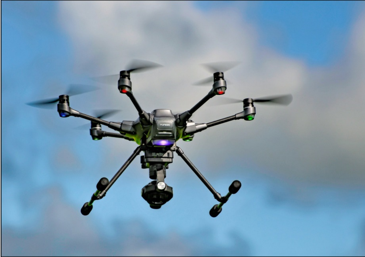
On take off, the undercarriage legs are down.
