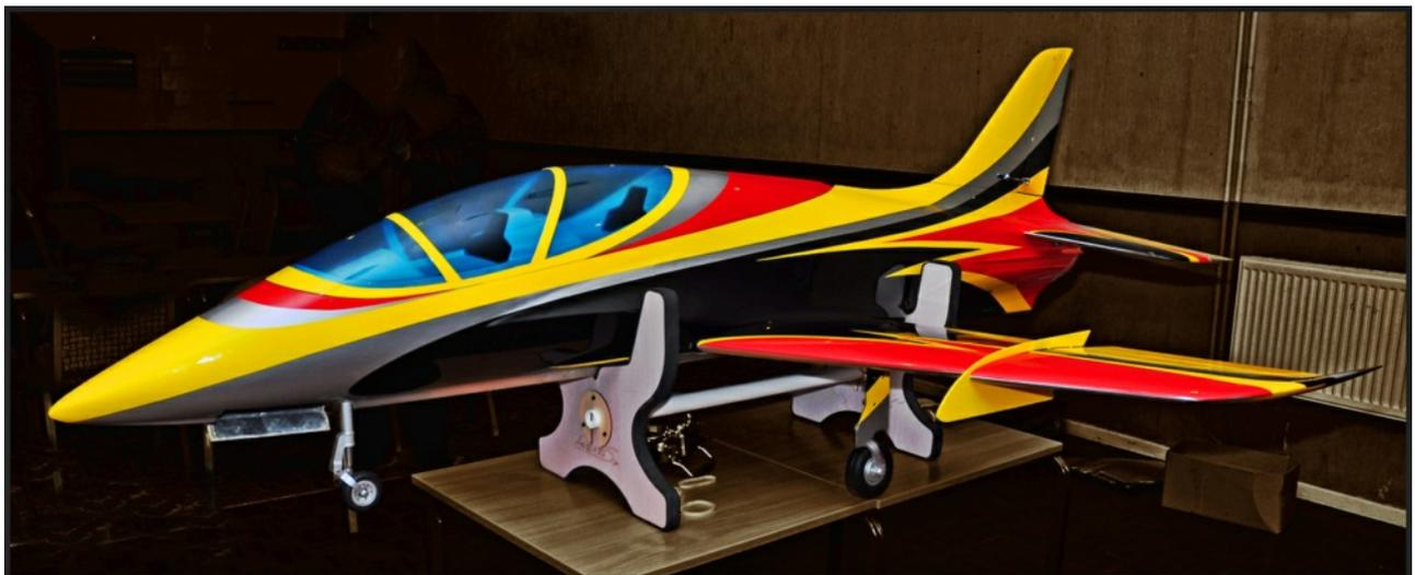
Mark Conlin brought his new Sebart model, the Avanti S. Another state of the art sleek jet but this time with vectored thrust. Mark said that it had presented many problems in mounting the jet engine - he had to make up jigs to be able to correctly align the motor within the very cramped space available. What he described to us sounded to have been a bit of a nightmare.
