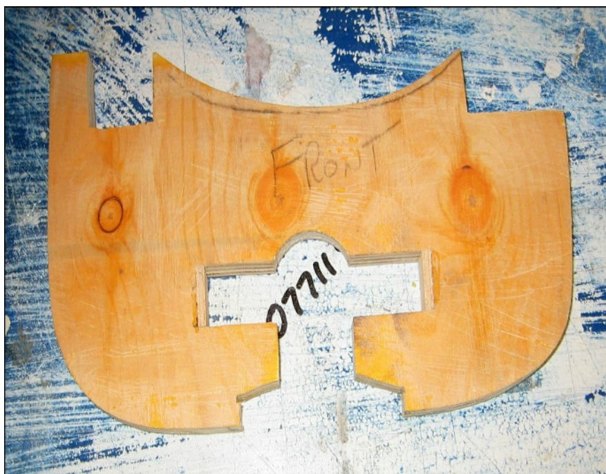
The new Birch ply formers cut out from the templates.
