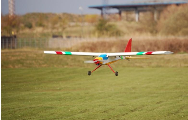
*This was my first conversion to electric - the Uno Wot. The motor produces 530 watts on 3 cell with a 12" x 6" prop. On 4 cell, it flies better than it ever did as on i.c.*
