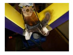
minor structural damage. Turns out that the temperature sensor's ability to detect changes quickly enough had reduced to the point where the engine management system kept demanding more fuel. i.e. it flooded and ignited!
